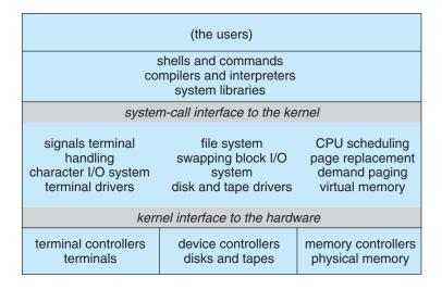
Figure A.2 4.4BSD layer structure.
