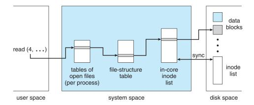
Figure A.7 File-system control blocks.
