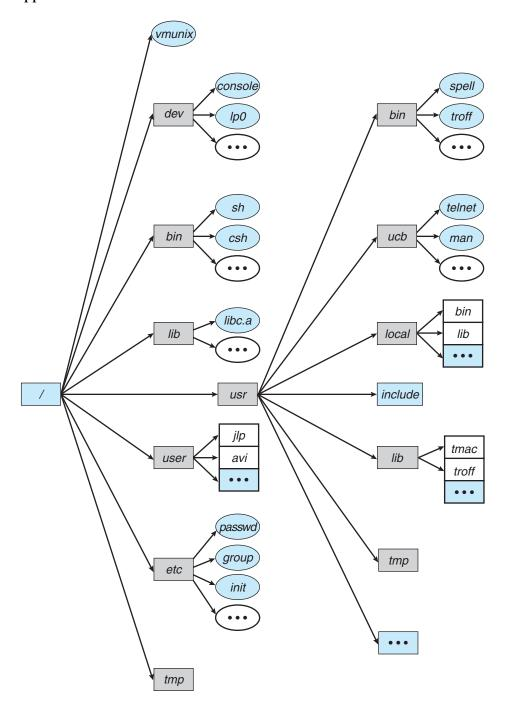
**Figure A.3** Typical UNIX directory structure.
