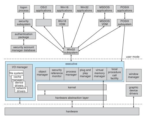
Figure C.1 Windows block diagram.
